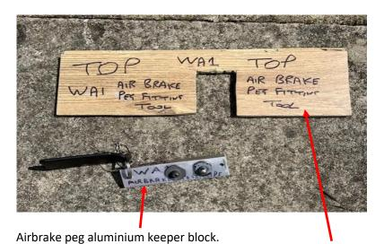
Wooden Block (Airbrake fitting tool) to hold A/B lever away from fuselage to allow room to fit the peg and block the slot below to prevent the peg falling below the seat pan.
